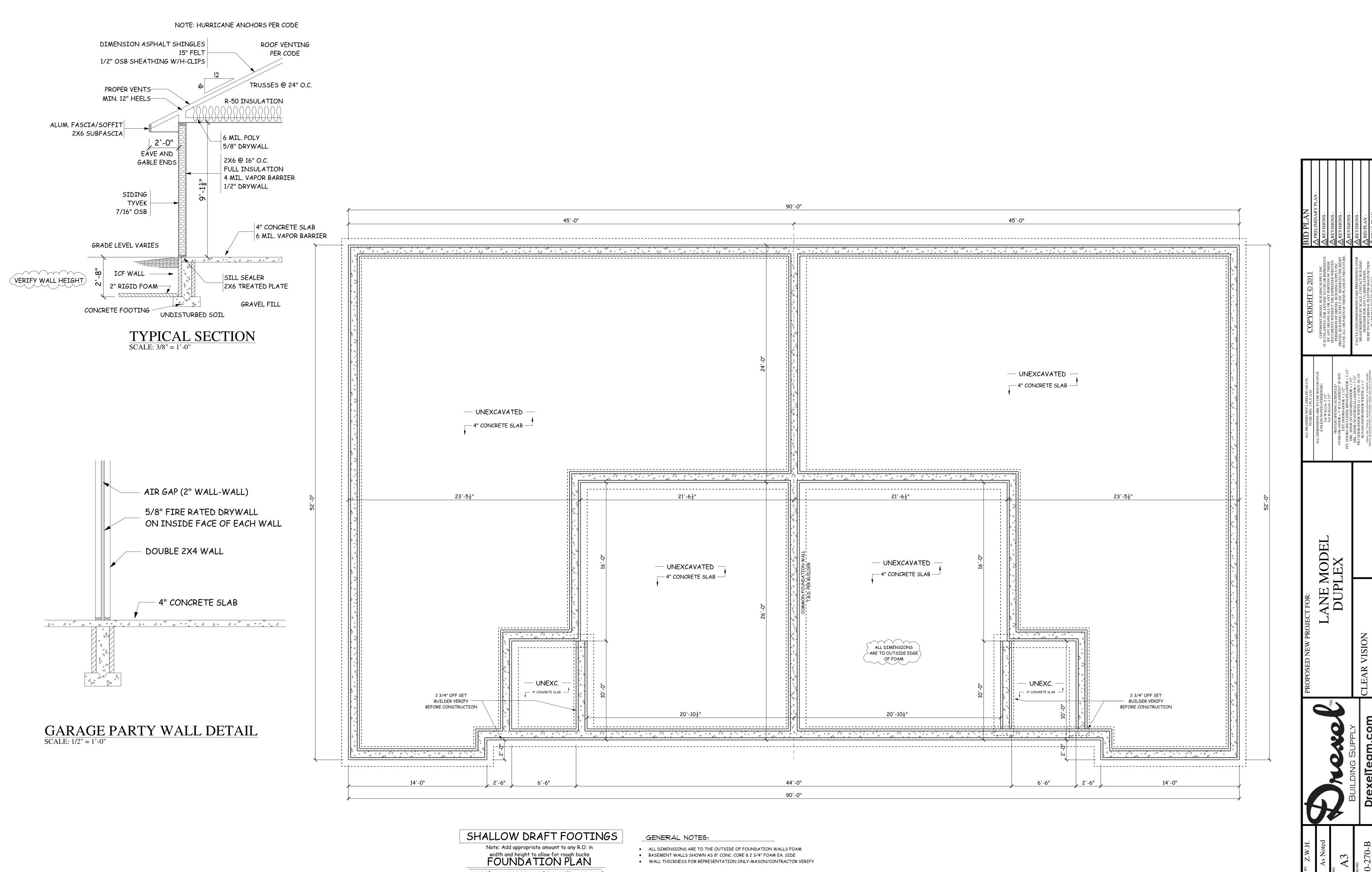
NOTE: MASON TO LOCATE PILASTERS AND SIZE FOOTINGS PER CODE & SOIL CONDITIONS
