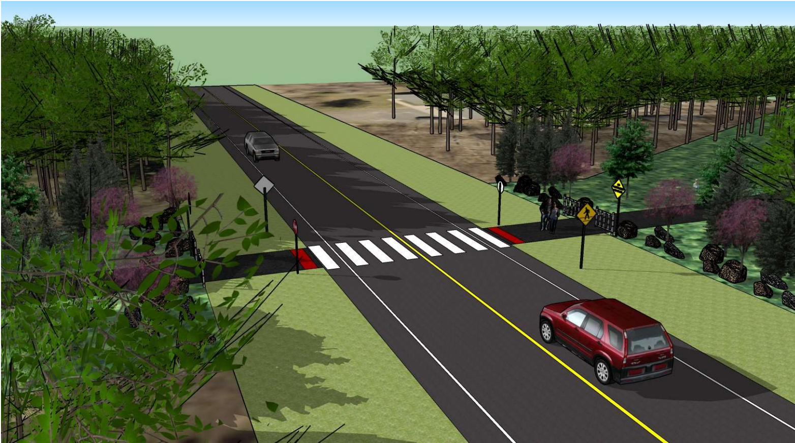
Road Crossing With Painted Crosswalk And Trail Crossing Signage
